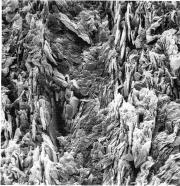
FIGURE 17-9 Scanning electron micrograph of domainal slaty cleavage from Upper Ordovician Martinsburg Slate near the Delaware River, Pennsylvania. Spacing between cleavage planes (strongly oriented narrow zones) is about 20 \mu\text{m} . (From Tectonophysics , v. 82, B. G. Woodland, p. 89-124, © 1982, with kind permission from Elsevier Science Ltd., Kidlington, United Kingdom.)
