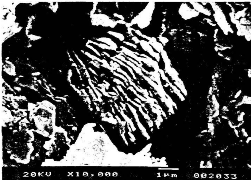
Figure 4B SEM micrograph of Mae Moh interburden mud rock showing "stack" or sheet-like structure of kaolinite. (Sample no. LM 4459C, IB. PT. Q2-Q3 192.5-193 m)
