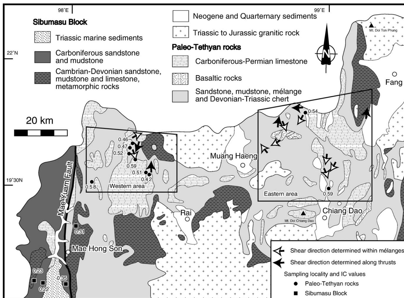
**Fig. 10.** Illite crystallinity values plotted on a simplified geological map of the Inthanon Zone. Black circles indicate sample localities within the Inthanon Zone; black squares indicate sample localities within the Sibumasu Block; the accompanying numbers are IC values ( $\Delta^{\circ}2\theta$ ). The shear directions presented in Fig. 9 are plotted on this map.
